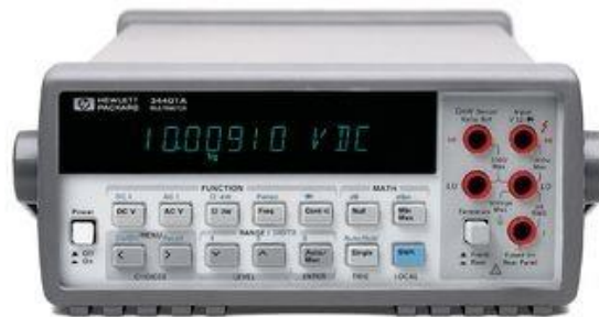
Fig.2 HP34401A (Located in E80 lab and VLSI lab)
